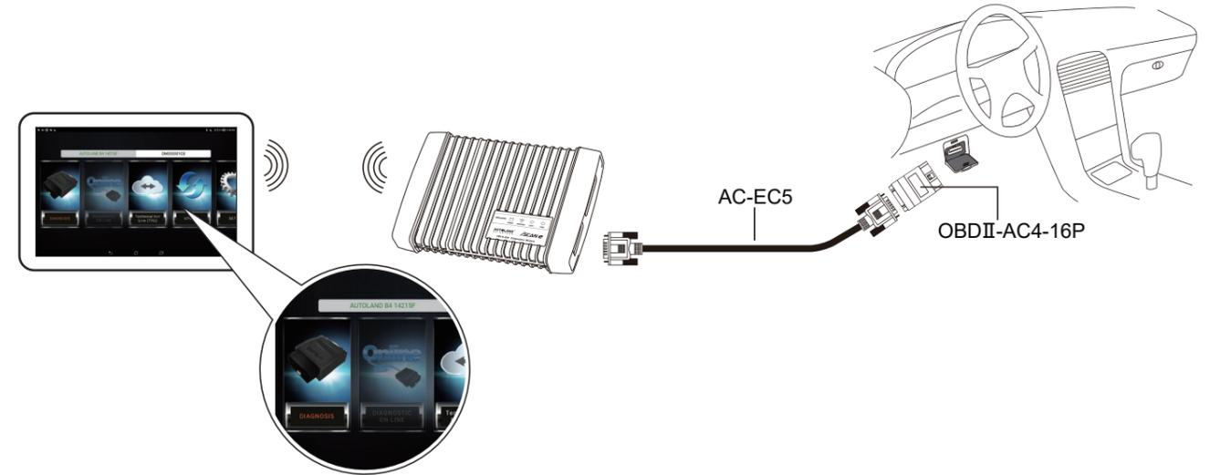
1. Connect OB15-DM to the vehicle with AC-EC5 & OBD-II adaptor.
