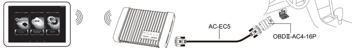
4. iSCAN-e system automatically searches and pairs to OB15-DM's Bluetooth.
